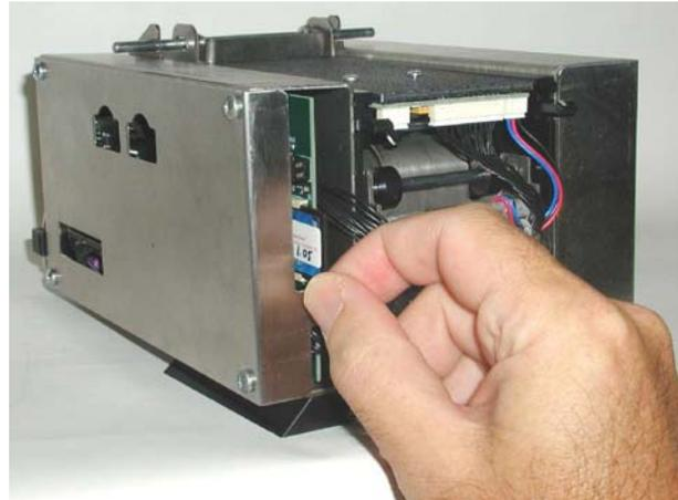
Follow the simple procedure below whenever you receive a “Flash” memory stick for updating the program in your System 600EF Note Acceptor.
